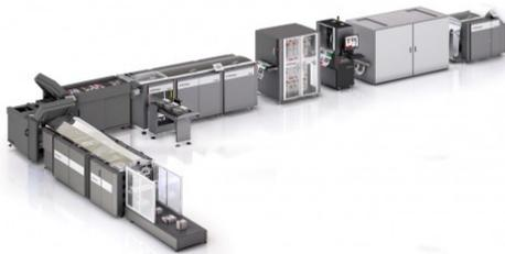
**Libra SR:** TecnaU adds to its Libra book-block making family with the introduction of the Libra SR system for short-run production of book blocks behind high-speed web-fed inkjet printers. Libra SR is based on TecnaU's established Libra One system which incorporates fully dynamic cutting, perforating and folding modules to
